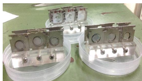
Fig. 3: Prepared ^{124}\text{Sn} (enriched) targets on Al-backing by vacuum evaporation method.
