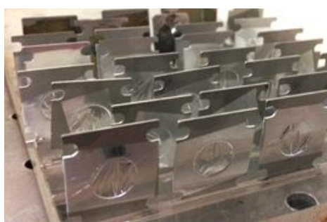
Fig. 1(c): Fabricated thin Al-catcher foils at Target Lab, IUAC.
