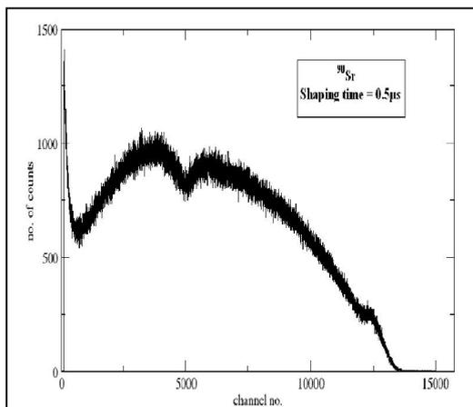
**Fig. 2** Beta ray spectrum of  $^{90}\text{Sr}$  source (at shaping time 0.5 $\mu$ s)
