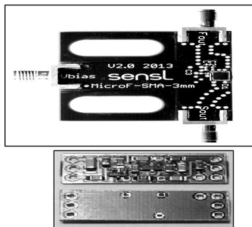
**Fig. 1** Advanced SiPM-Preamplifier combination for detector testing
