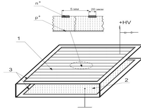
**Fig. 2:** Schematic diagram of planar germanium detector with orthogonal strips. 1) Charge pickup strips. 2) Sensitive germanium volume. 3) Guard electrodes in the anode and cathode planes. Zoomed portion of pickup strips is shown in the inset.
