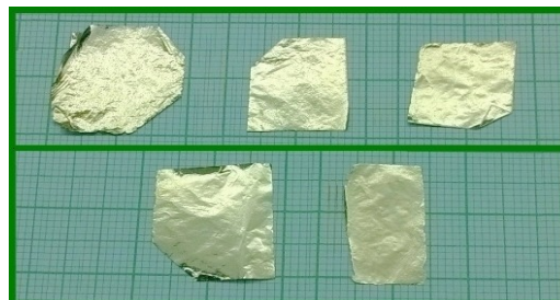
Fig. 3 Thin ^{176}\text{Yb} foils of various thickness
