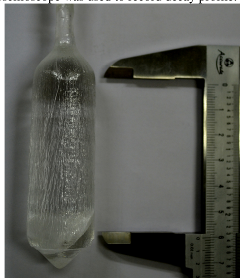
Fig. 1 Single crystal ingot of YAP:Ce
