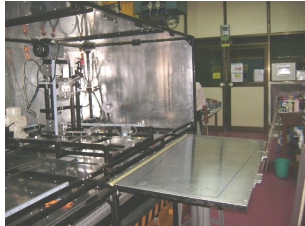
Fig. 4 : An intense x-ray source with x,y,z positioner, inside a lead (1mm thick) cubicle for illuminating and characterizing GE1/1 and similar sized GEM detectors at NPD-BARC
