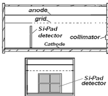
Fig.1: Schematic diagram of the hybrid detector telescope.
