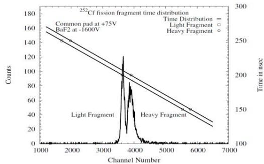
Fig.3 Time distribution for the fission fragments measured by BaF<sub>2</sub>-Silicon setup.
