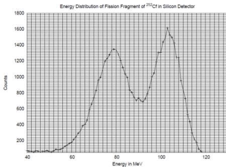
Fig.2 Energy distribution for fission fragments measured by Si-pad detector.
