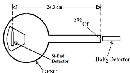
Fig.1 Schematic diagram of Time of Flight setup.
