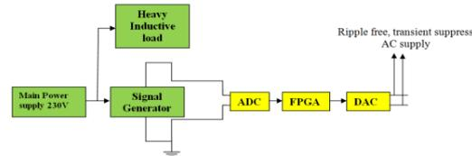
**Fig.4** Testing set up
