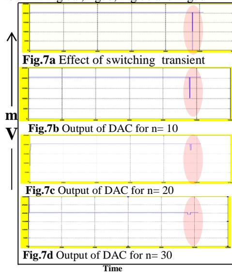
It is observed that switching on heavy inductive load drops the main supply significantly which in turn introduced transient/glitches in other systems connected to mains. Results obtained in Fig.5(a,b,c,d), and Fig.7(a,b,c,d) clearly indicates that if order of moving average filter increased there is significant suppression of any glitch or switching transients . Moreover for higher orders, signal to noise ratio improves considerably as shown in Fig.6b.
