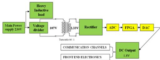
**Fig.3** Layout of Detector power supply
