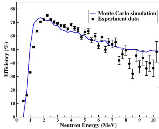
**Fig. 2** Variation of Neutron detection efficiency as a function of energy
