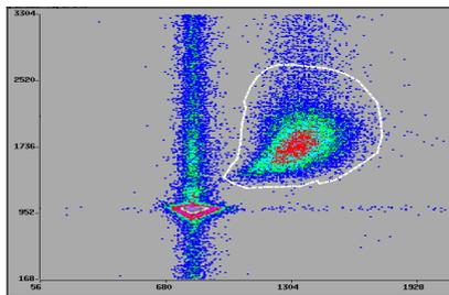
**Fig. 1** Two dimensional plot showing PSD against TOF. Events in the marked region are neutrons
