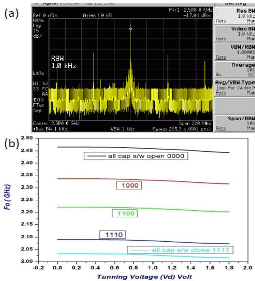
Fig. 3 (a) Frequency Spectrum (b) Tuning test
