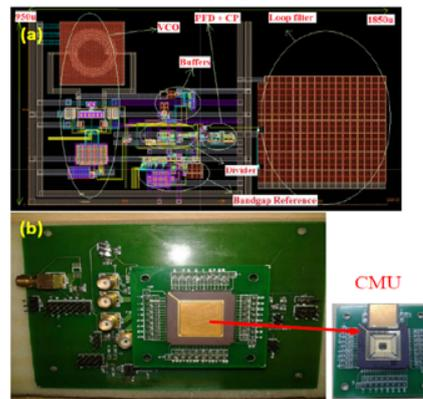
Fig. 2 (a) Layout of PLL (b) Test setup for developed CMU
