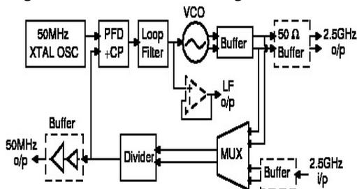
Fig. 1 Block diagram of clock multiplier unit
