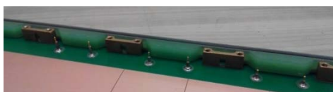
Fig. 3 picture of the HV contact pins soldered on the PCB.
