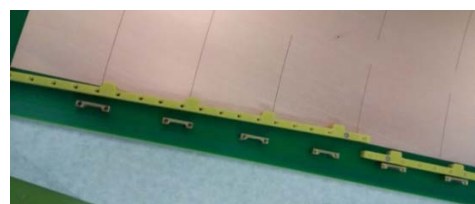
Fig. 2. Picture of the brass supports and inner frames being fixed on the PCB plane.
