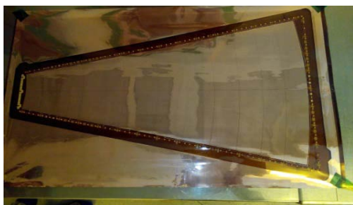
Fig. 1 Picture of the trapezoidal shaped GEM foil. The raw materials available to produce these foils have a maximum width of about 60 cm,
