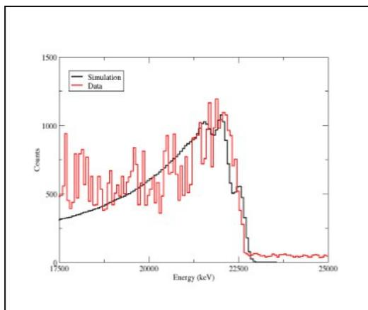
Figure2. The measured energy spectrum for 22.5MeV  $\gamma$ -rays produced in the  $p(^{11}\text{B},\gamma)^{12}\text{C}$  reaction. The solid line is the GEANT4 simulation of the spectrum.
