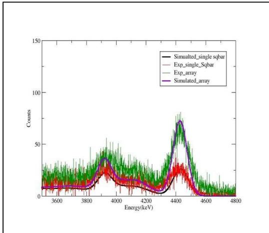
Figure1. Measured energy spectrum of 4.43MeV  $\gamma$ -rays from the  $^{241}\text{Am}-^9\text{Be}$  source in the  $\text{LaBr}_3:\text{Ce}$  detector. The solid line is the GEANT4 simulation of the spectrum.
