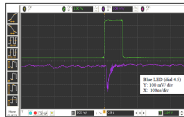
Fig 3: Oscilloscope response of the novel photo structure in 0.35 um CMOS process.
