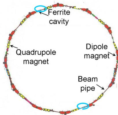
Fig. 2 Major components in SIS ring at GSI.
