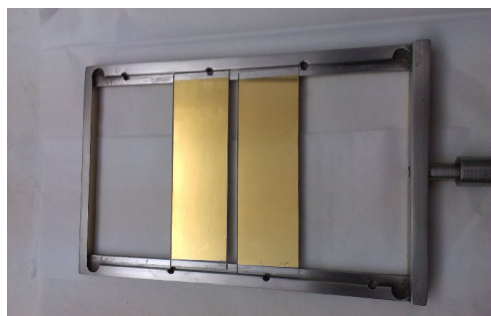
Fig. 1: Substrate after the deposition of ^{197}\text{Au} on glass substrate with soap solution as parting agent.
