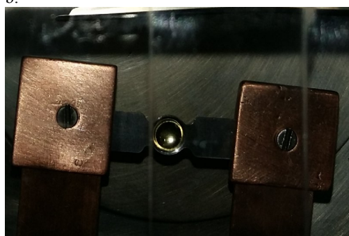
Fig. 2 (a): High Vacuum Evaporation setup for the evaporation of target material with Dimple boat.
