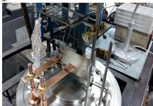
Fig. 1: Substrate after the deposition of ^{197}\text{Au} on glass substrate with soap solution as parting agent.
