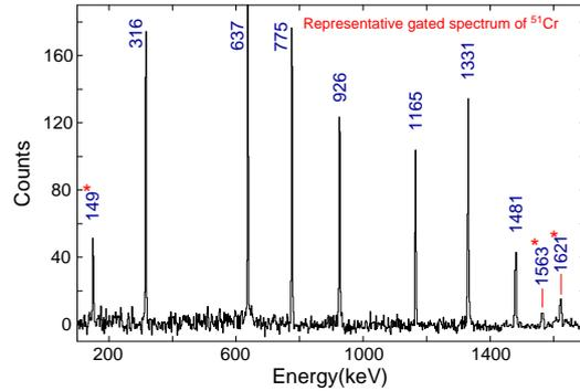
FIG. 2: Representative gated spectrum of  $^{51}\text{Cr}$  with double-coincidence gates on 1747 keV transition and one of the transitions from the list L: 1165, 1481, 316, 775, 926, 637, 1563 keV. The newly observed transitions are marked with “\*”.
