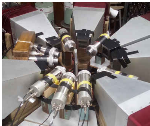
FIG. 1: Set-up used for angular correlation measurement for ^{150}\text{Sm} \gamma rays.
