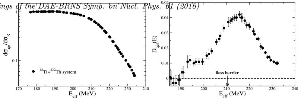
FIG. 2: Final experimental QE excitation function (left) after smoothing and the corresponding barrier distribution (right) for the  $^{48}\text{Ti}+^{232}\text{Th}$  system.
