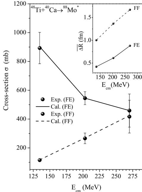
FIG. 1: The calculated FE and FF channel cross-sections for hot and rotating CN  $^{88}\text{Mo}^*$ , formed in the reaction  $^{48}\text{Ti} + ^{40}\text{Ca} \rightarrow ^{88}\text{Mo}^*$  at two  $\overline{\Delta R}$ -values for  $E_{cm} = 134.7, 203$  &  $270$  MeV is compared with the experimental-data [1] and the inset shows the  $\overline{\Delta R}$ -values required at different center of mass energies for FE and FF channels.
