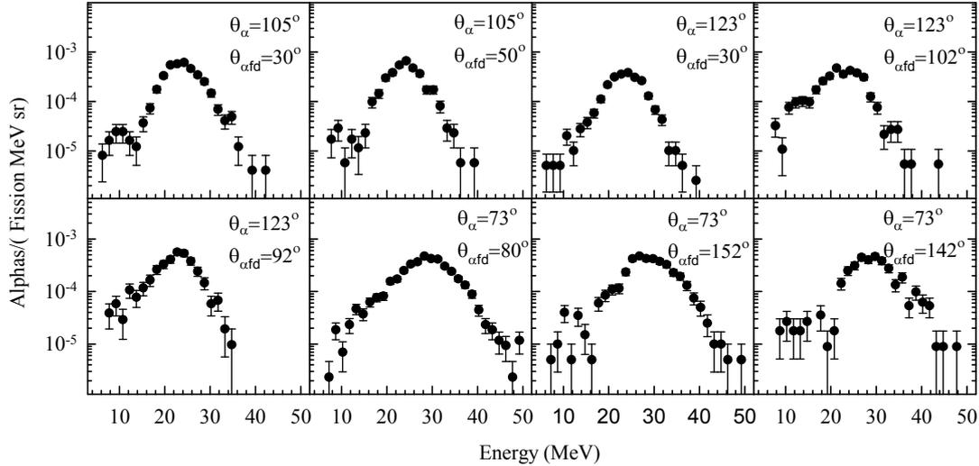
FIG. 2: The  $\alpha$ -particle multiplicity spectra for different combination of laboratory angles of CsI(Tl) detectors with respect to beam direction,  $\theta_\alpha$  and detected fission fragments,  $\theta_{\alpha fd}$ .
