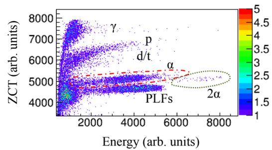
FIG. 1: A two dimensional plot of zero cross over (ZCT) versus energy from a CsI(Tl) detector at laboratory angle of 123° for different particles produced in the  $^{13}\text{C} (75 \text{ MeV}) + ^{232}\text{Th}$  reaction.
