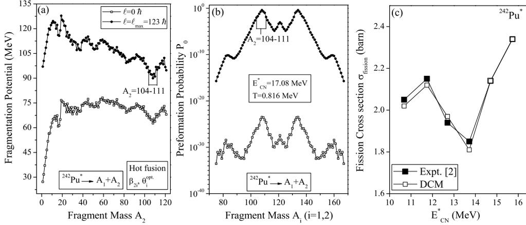
FIG. 1: (a) The fragmentation potentials for the decay of  $^{242}\text{Pu}^*$  plotted at extreme values of angular momentum for  $\beta_2$  deformed choice, at neck-length value of  $\sim 1.23$  fm. (b) Same as (a) but for preformation probability  $P_0$ . (c) Comparison of the DCM based fission cross-sections with measured data [2] over a wide range of excitation energies.
