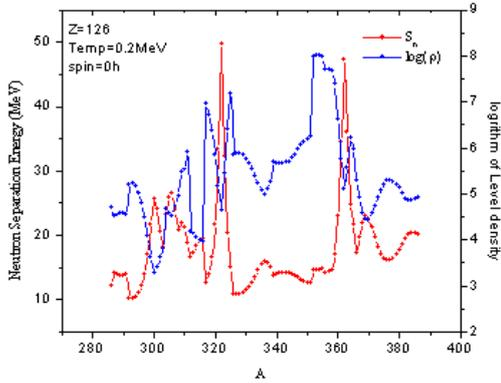
**Fig. 1** Neutron separation energy and level density of Z=126 with a range of neutron. The drop in level density indicates the possible neutron shell closures.
