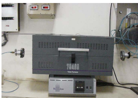
FIG. 3: Tube furnace used for annealing at IUAC, New Delhi.
