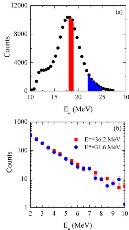
**Fig. 3** (a)  $\alpha$ -particle energy spectrum in centre of mass with two energy cuts shown by filled area. (b) Neutron energy spectra corresponding to two  $\alpha$ -particle energy cuts shown in (a).
