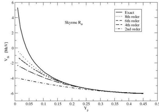
**Figure 2.**  $V_{th}$  as a function of the proton fraction  $Y_p$  at density  $\rho = 0.08 \text{ fm}^{-3}$  for exact, 8<sup>th</sup> order, 6<sup>th</sup> order, 4<sup>th</sup> order and 2<sup>nd</sup> order Taylor expansion for the EOS of Skyrme interaction using  $R_\sigma$  set.
