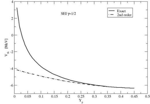
**Figure 1.**  $V_{th}$  as a function of the proton fraction  $Y_p$  at density  $\rho = 0.08 \text{ fm}^{-3}$  for exact and 2nd order PA for the EOS of SEI.
