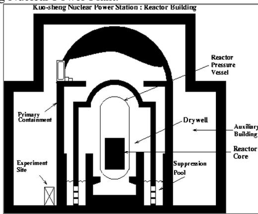
FIG. 1: Schematic side view of the Kuo-Sheng Nuclear Power Plant Building, indicating the experimental site. The reactor core-detector distance is about 28 m [2].
