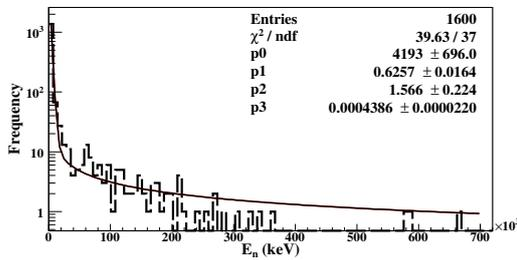
FIG. 1: The energy distribution of neutrons from 10 GeV muons after propagating through rock.
