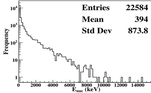
FIG. 2: Distribution of kinetic energy of all the recoiling nuclei of GGAG.
