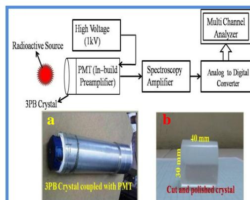
**Fig.1** Schematic diagram of experimental setup (a) 3PB crystal coupled with PMT (b) cut and polished crystal grown by SR technique
