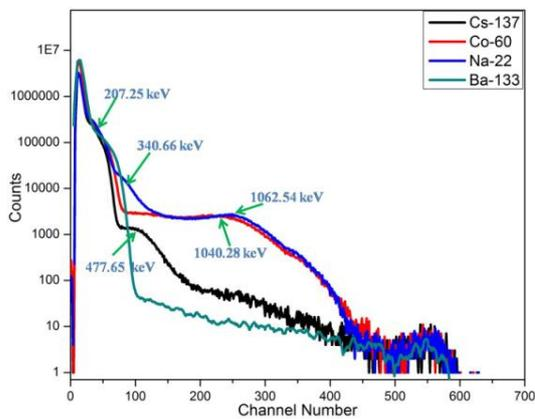
**Fig.2** Energy spectrum of 3PB single crystal with different radioactive sources
