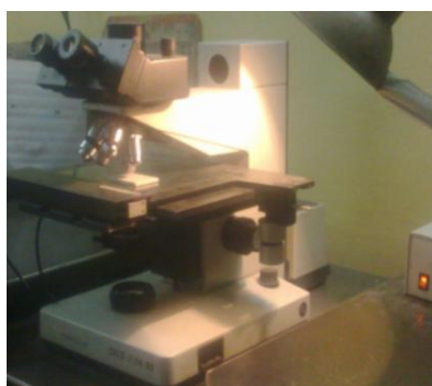
FIG. 1: Photograph of Olympus BH-2 binocular microscope having 100X objective and 15X eyepieces.
