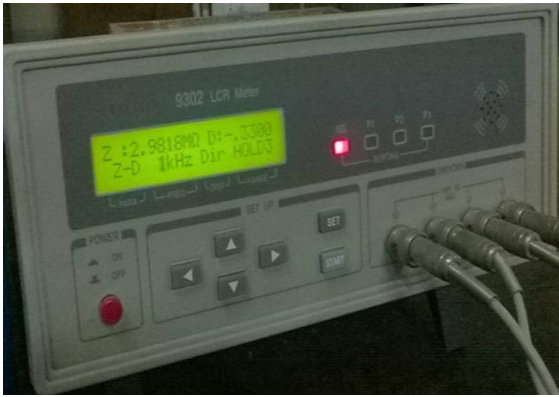
FIG. 3: 9302 LCR meter for measurement of capacitance (C), inductance (L) and impedance (Z).
