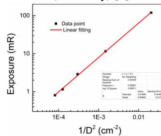
**Fig.5.** Estimated exposure of FXR with  $1/D^2$
