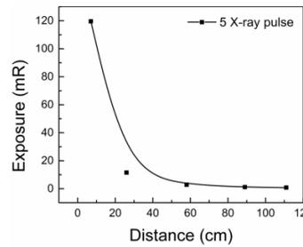
**Fig.4.** Measured doses for 5 X-ray pulses for the FXR at different distances from the source window.
