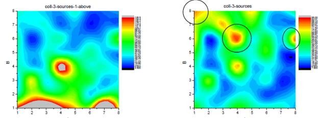
**Fig. 3** MAPMT output showing the spatial position of three point source using a single slab of CsI:TI crystal along with lead collimator.
