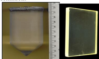
Figure 1: Photograph of CsI:Tl (a) single crystal ingot (b) plate of size 49 mm x 51 mm x 6 mm under UV illumination.
