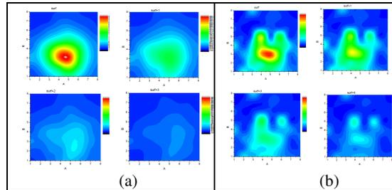
**Fig. 2** MAPMT output showing the displacement of radiation source away from the MAPMT without any collimator (a) by using pixilated crystals (b) using a single crystal. (Top left data source at 2 mm distance from device, top left 5 mm, lower left 10 mm, lower right 20 mm)
