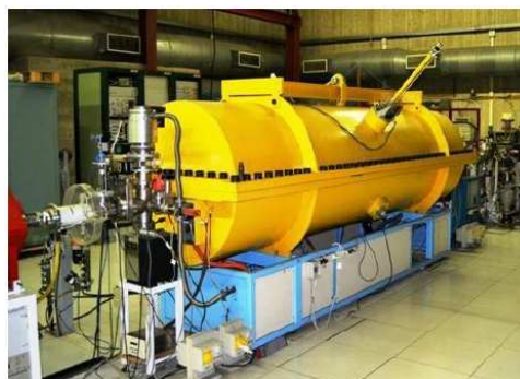
Fig.1 Tandem accelerator (TTT-3) at University of Naples Federico II. It is horizontally installed having maximum terminal voltage is 3.3MV.
