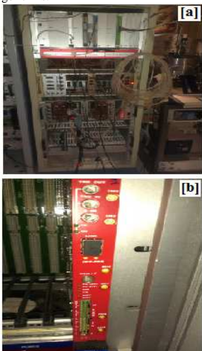
Fig.2 [a] The data acquisition system and the connected Fiber optics with the High voltage Power supply.[b] The used eight channel CAEN V1720 Digitizer.
