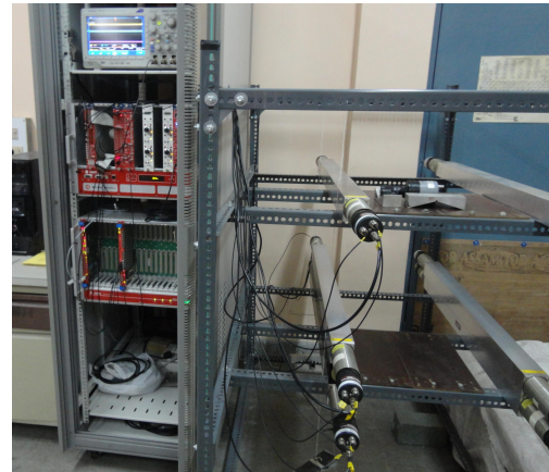
FIG. 1: The setup for the muon measurements.
