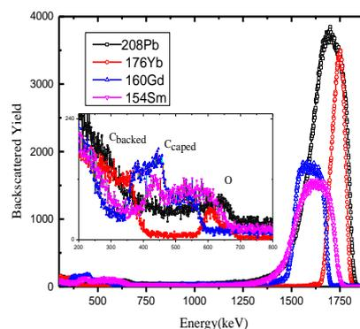
Fig. 1. RBS Spectra of 154Sm, 160Gd, 176Yb and 208Pb target sample.
