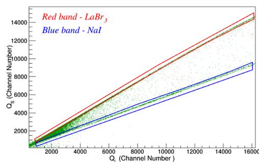
FIG. 1: Neutron gated  $Q_L$  vs  $Q_S$  Spectrum for <sup>252</sup>Cf source.
