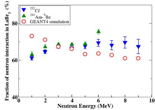
FIG. 3: Fraction of neutron events in  $\text{LaBr}_3$  with respect to total events in Phoswich detector. The neutron energies are with uncertainty of  $\pm 0.5$  MeV
