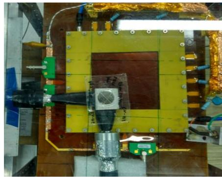
Fig. 1 Triple GEM detector lab setup.
