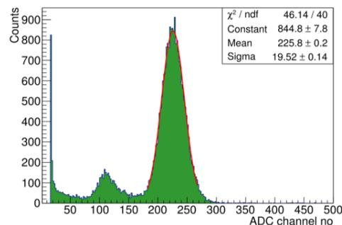
Fig. 2 <sup>55</sup>Fe spectrum of a triple GEM detector.
