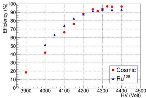
Fig. 5 Efficiency variation as a function of HV for cosmic muons and  $^{106}\text{Ru}$ -Rh source.
