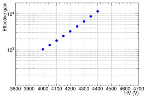
Fig. 3 Gain variation as a function of HV.
