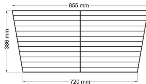
Fig. 1 Dimensions of OROC3 GEM foil.
