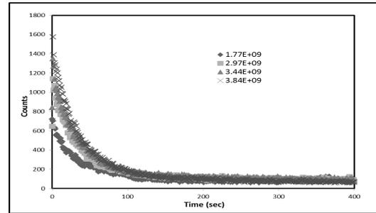
Fig.2 Decay curves of 20nsec pulses for different yield.
