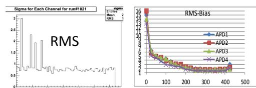
Fig. 2: Typical RMS values at 425Volts and variation of RMS with bias voltage
