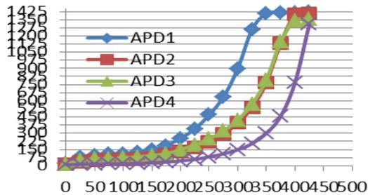
Fig. 3: ADC output vs bias voltage for different wavelengths
