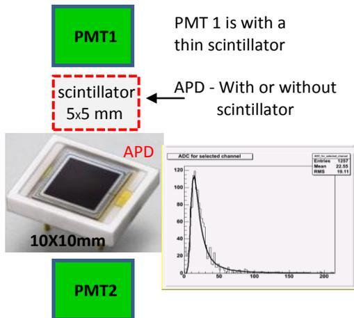
Fig. 4: Coincidence setup for tests with cosmic and Beta source
