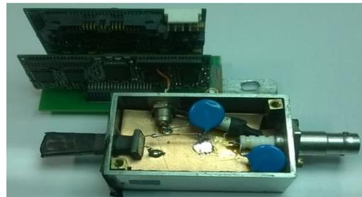
Fig. 4: Setup with APD coupled with Scintillator
