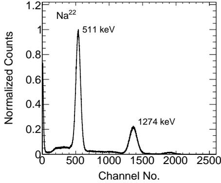
FIG. 2: Pulse height response of a BGO detector in the presence of  $^{22}\text{Na}$  source.
