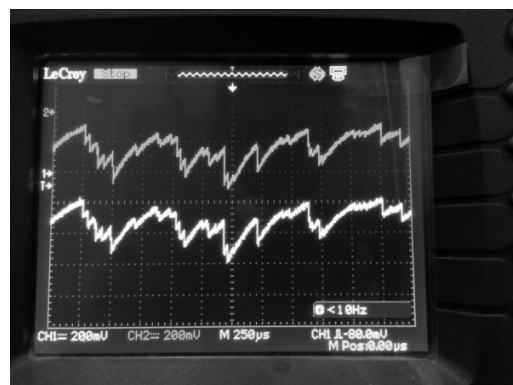
Fig. 3 Oscilloscope signal corresponding to one end each of X (bottom signal) and Y (top signal) anode chain.
