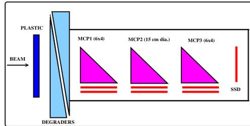
**Fig. 4:** Layout of detector system in CAVE'C'
