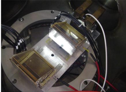
**Fig. 2:** Picture of MCP TOF system
