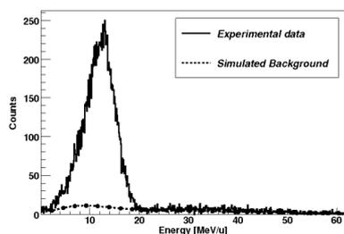
**Fig. 1:** Energy distribution of  $^{64}\text{Ni}$  ions after slowing down in Al degrader [2].
