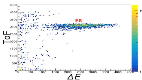
FIG. 1: The energy loss versus ToF spectrum for the reaction  $^{28}\text{Si} + ^{192}\text{Os}$  at 157 MeV beam energy.
