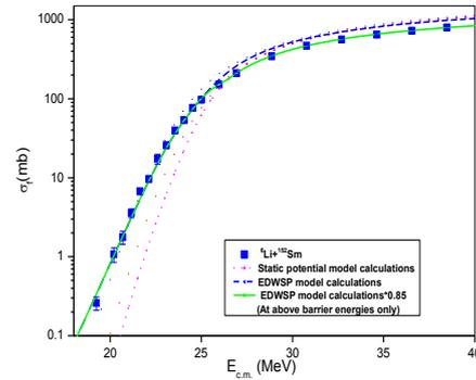
Fig.2. Fusion excitation functions of  ${}^6\text{Li} + {}^{152}\text{Sm}$  reaction obtained by using the static Woods-Saxon potential and the EDWSP model [3-5]. The calculational results are compared with the experimental fusion data taken from Ref. [2].
