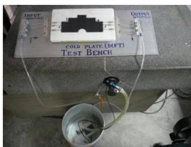
**Fig. 3** The prototype with water flow system
