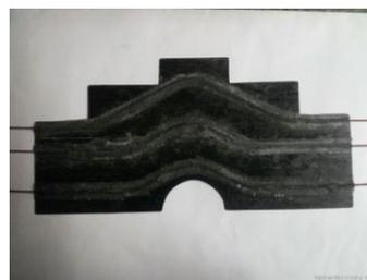
**Fig. 1** The water-cooling prototype for MFT
