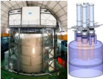
**Fig. 2** Photograph of LEGEND-200 and sketch of baseline cryostat design for LEGEND-1000.
