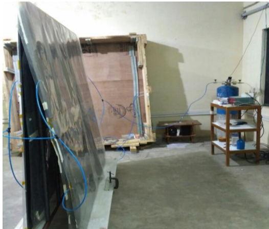
Figure 3: High Voltage Test stand for the RPC detector at IICHEP, Madurai.
