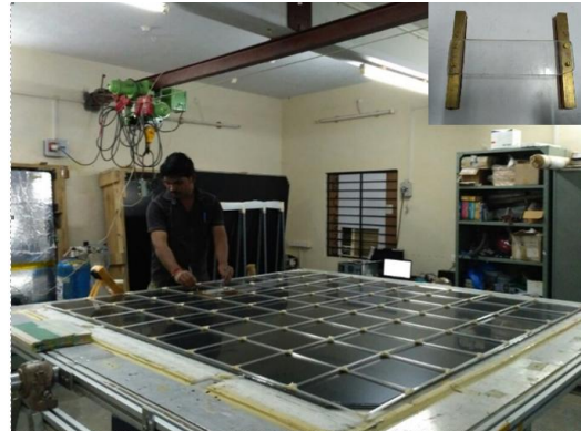
Figure 1: Surface resistivity measurement of graphite coated RPC detector's electrodes and inset picture is of the Copper Jig.
