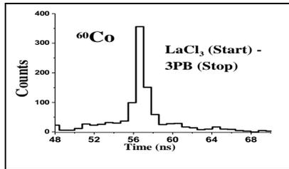
**Fig. 2** The prompt TAC spectrum with a  $^{60}\text{Co}$  source, without any selection in energy.
