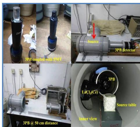
**Fig.1** Time of flight experimental setup
