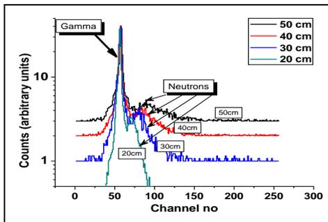
**Fig. 3** TAC spectra for distances 20 to 50 cm with 16 ns fixed delay in the stop signal. The spectra for different distances are shifted vertically to show the shift in neutron peak clearly.
