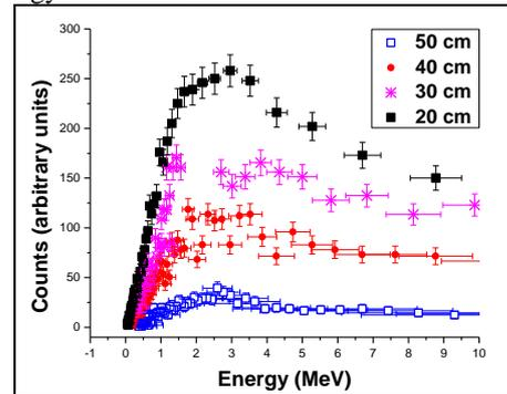
**Fig. 4** Neutron energy spectrum with varying distances.
